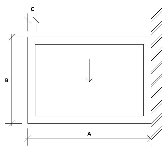
A = O/A Length from Wall to Outside Finished Curb (mm)
