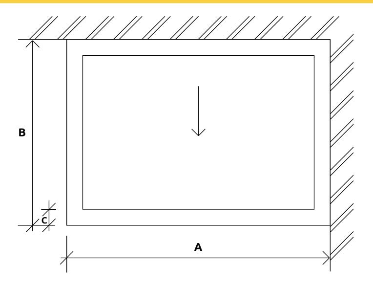
A = O/A Length from Wall to Outside Finished Curb (mm)
