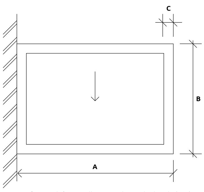
A = O/A Length from Wall to Outside Finished Curb (mm)
