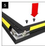
Ensure the mitred eaves ends are pressed up against each other now fix the cleats into the eaves beam using the M5 x 8mm fixings provided through the pre-drilled
