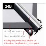
If positioned correctly the glazing end profile will extend beyond the centre point of the glass stop.
