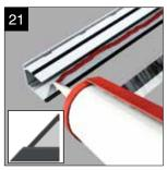
Using MS polymer seal underside of top face of glazing end profile as shown. Depending on the roof specification this can either be a PVCu or Aluminium profile. At hips these will be mitred and extend beyond the glazing. At transoms these will be square cut and extend beyond the glazing.
