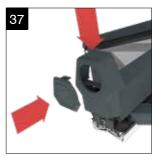
Fit end caps to rafters and push in the end cap infill.
