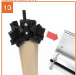
Ensure the assembled ridgeLOCK is Prop the ridge body, now attach the left propped throughout the assembly hand hip rafter by inserting the ridgeLOCK process. Fit each hip rafter to the tenons of the ridgeLOCK. Secure in place into pre drilled holes using M5 x 16mm screw in the upper hole and the M5 x 20mm screw in the lower hole
