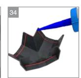
Apply a small bead of MS polymer to the inside of the external cover (as shown) around where the part meets the glazing rafter top caps and the ridge top cap.
