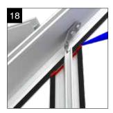
Seal the area where the hip rafter abuts the iack rafter as shown above
