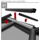
Ensure the weathering shield is in place then fit the ridge top cap, ensuring that the top cap clips are evenly spaced. Push down along the length to check the top cap is fully engaged. Now fit the rafter top caps using the same method, taking care not to damage the finish of the ridge top cap.
