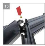
If the project contains central rafters between the hips. Position the rafter between the two hip rafters, secure using the 30mm hex bolt and flanged nut provided.
