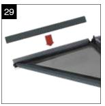
Work your way around the roof and fit the rafter top caps.
