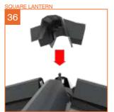
Clip the external cover on top of the ridgeLOCK and assembled bars. Ensure the clip hole in the cover is aligned with the corresponding ridgeLOCK clip feature.
